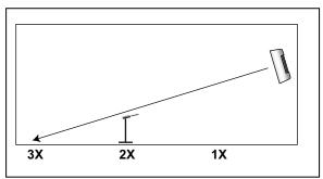
Figure 10 - Typical Measurement Microphone Placement
